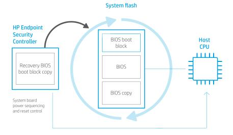
Figure 1 illustrates the firmware integrity verification process. Once the HP ESC authenticates and starts executing the HP Sure Start firmware, that firmware uses the same strong cryptographic operations to verify the integrity of the system flash BIOS boot block. If a single bit is invalid, the HP ESC replaces the system flash contents with its own copy of the HP BIOS boot block that is stored within an isolated non-volatile memory (NVM) dedicated to the HP ESC.
